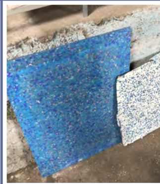
Shredded plastic put into a tray, then to the melting oven, which creates a big plastic slab.
