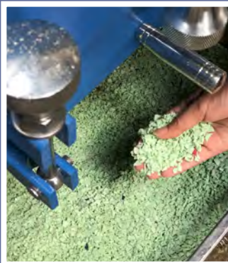
All clean plastic are divided by colors and then shattered into small pieces.
